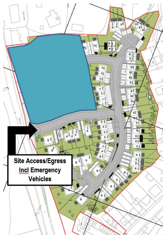
Fig. 4. Blue block area denoting site compound/welfare/material storage/contractor parking
