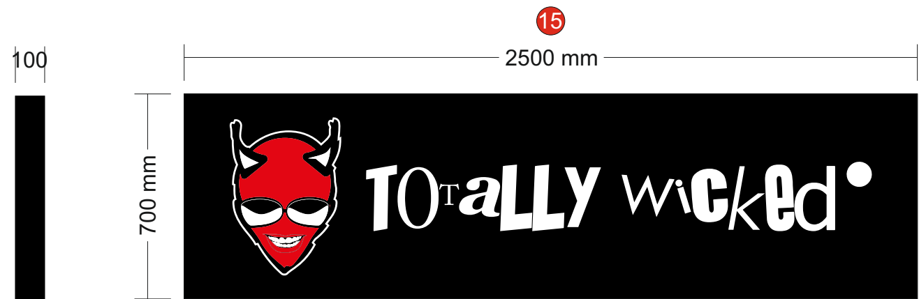
1 off Totally Wicked brand badge made from 2mm Aluminium with logo & text stencil cut away from it coated Black RAL 9005 with applied digital print graphic ( devils head ). Brand badge internally illuminated via 6500k cool White LEDs & power supply to suit mounted to back tray.
