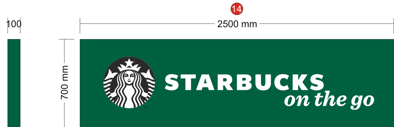
1 off Starbucks brand badge made from 2mm Aluminium with Starbucks logo & text stencil cut away from it coated Green NCS 5040g matte with applied gloss black Starbucks graphic. Brand badge internally illuminated via 6500k cool White LEDs & power supply to suit mounted to back tray.
