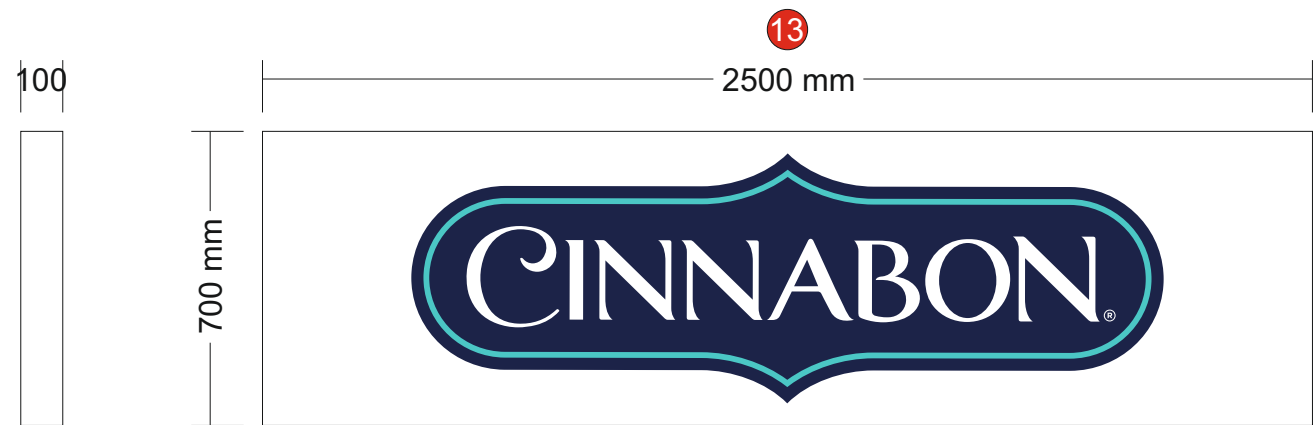
1 off Cinnabon brand badge made from 2mm Aluminium with Cinnabon logo stencil cut away from it & backed up with 3mm 050 Acrylic faced in digital print printed on back lit settings matt UV laminated. Coated White RAL 9003 internally illuminated via 6500k cool White LEDs & power supply to suit mounted to back tray.
