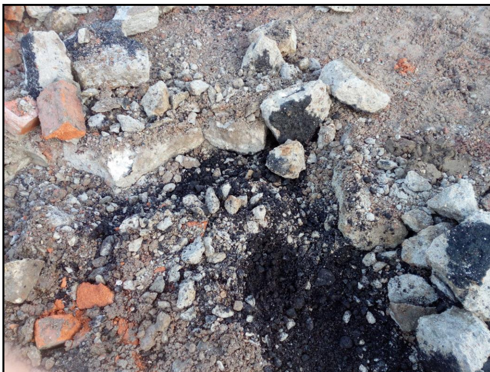
Plate 6.1. Example of black ashy made ground from beneath former floor-slab
