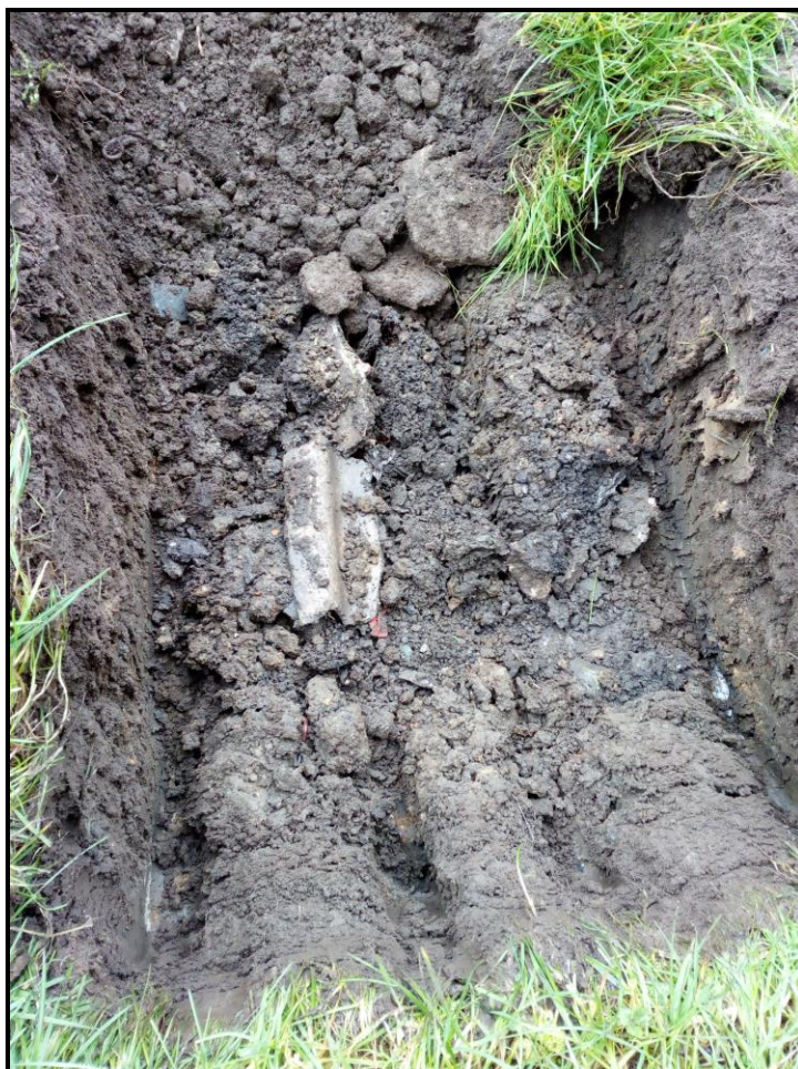
Plate 5.1. Corrugated Asbestos Cement, TP03, 0.4m
