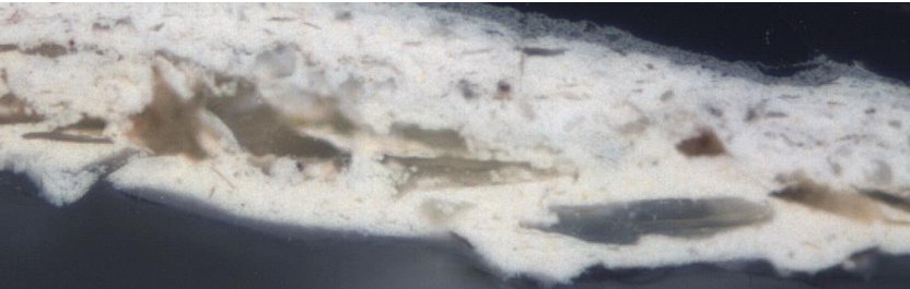
Textured paint layer containing large chunks of silica resting over a light stone coloured base coat
