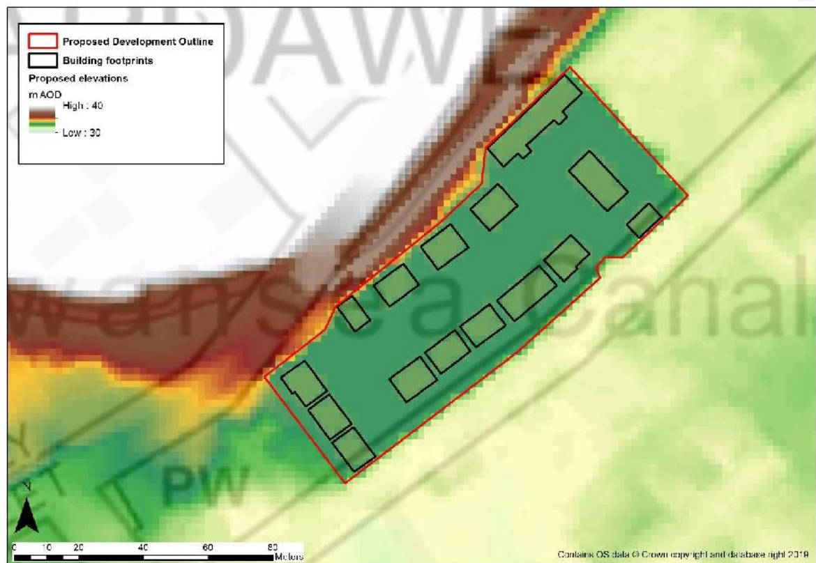
Figure 4-3: Post-development site layout and levels
