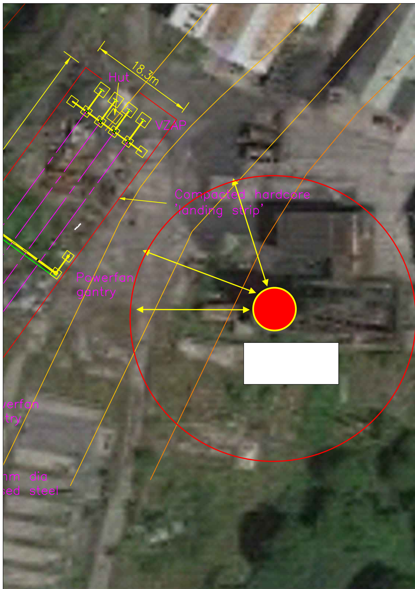
FIGURE 10 DETAIL OF ZIPLINE CONSTRUCTION ON AERIAL PHOTOGRAPH. ALL STRUCTURES ARE GREATER THAN 20m FROM SHAFT
