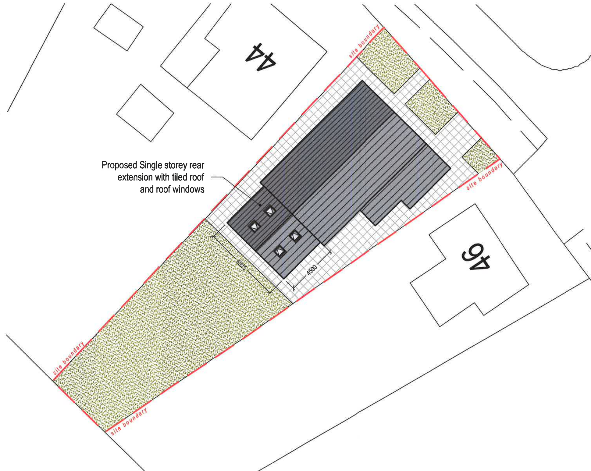
PROPOSED SITE PLAN Scale 1:200
