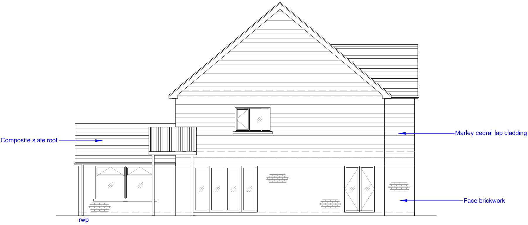
SIDE ELEVATION (North East)
