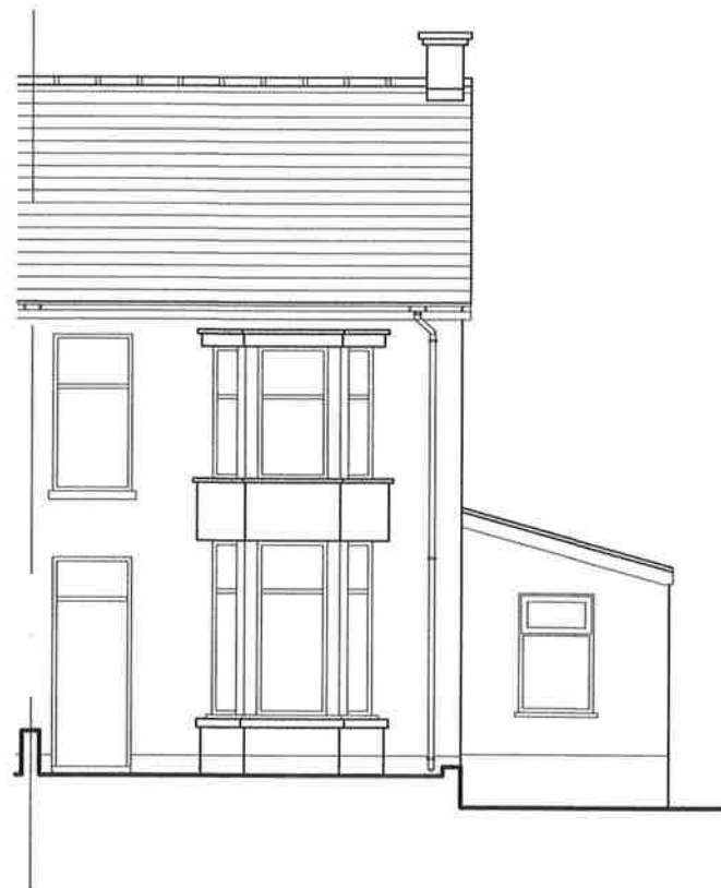
Existing Front Elevation
