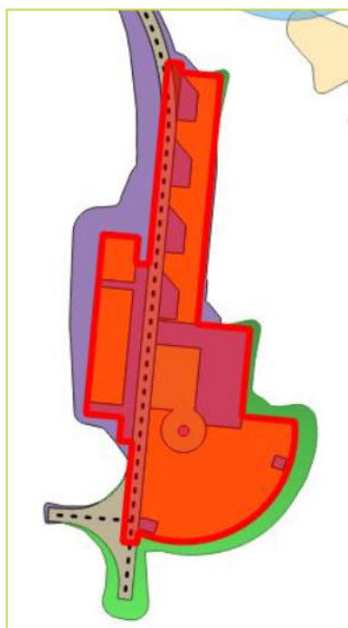
Image 6.1: Turbine hardstanding contributing areas
