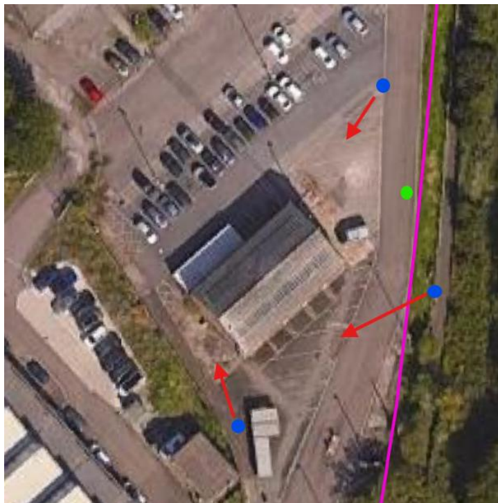
Figure 2 Survey coverage plan showing thermal camera positions and viewing directions, surveyor position and acoustic detector coverage.
