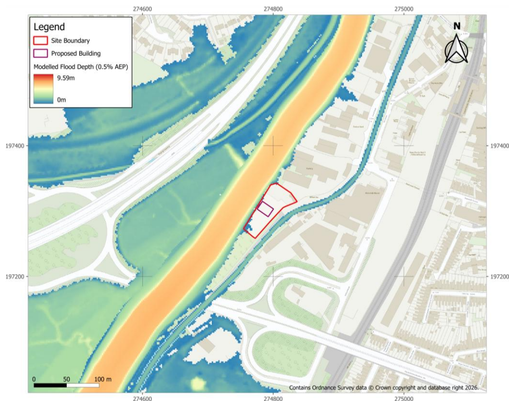
Figure 4-4 - Post-Development Flood Depths. 0.5% AEP. Tidal.
