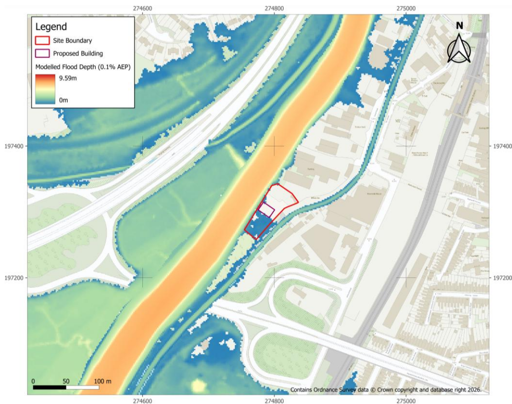
Figure 4-6 - Post-Development Flood Depths. 0.1% AEP. Tidal.
